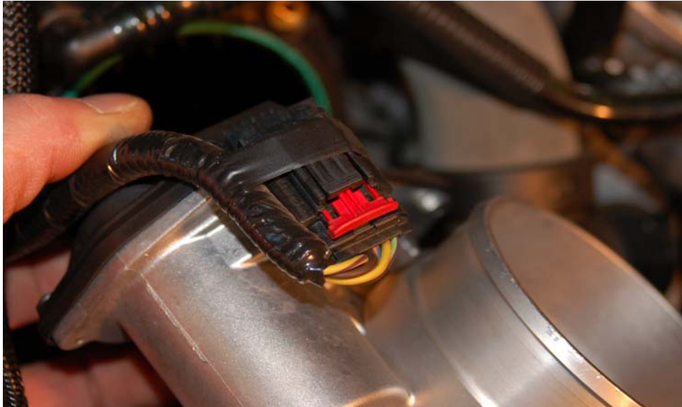
Fig. 4 Disconnect throttle body motor control plug. Slide red tab out, then push on black tab.
