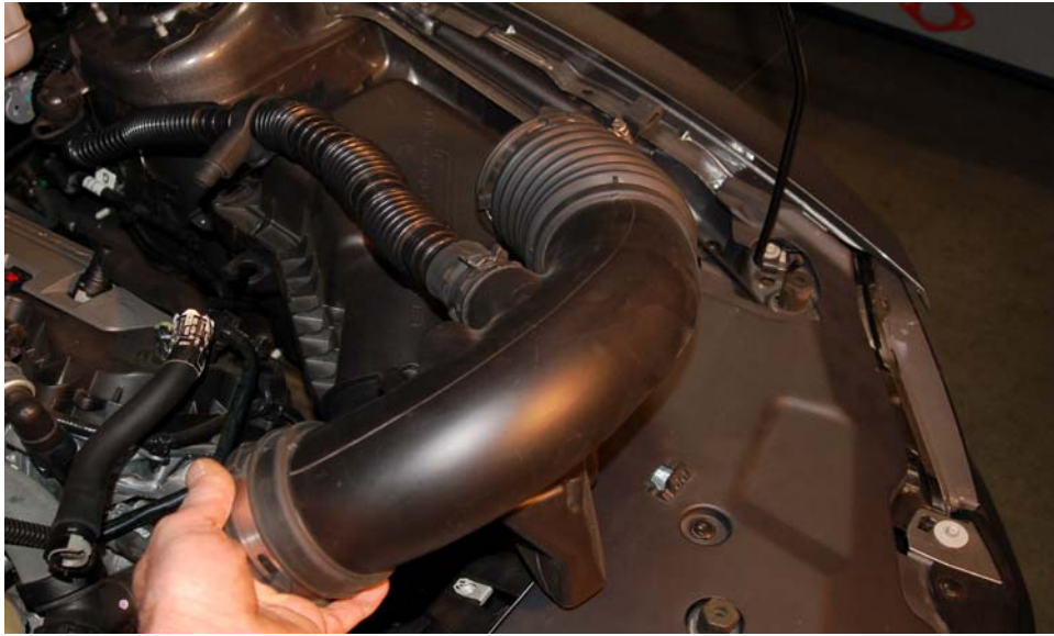
Fig. 3 Set air inlet tube aside, out of the way.
