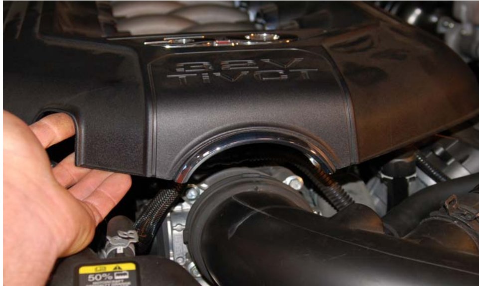
Fig. 1 Removing engine cover to access throttle body.
