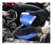
Remove the Mass air sensor from the stock air box and install it into the BBK Cold Air Tube using the supplied hardware. (The sensor will only go in one way) Install the angled BBK coupler with the vacuum port in it onto the throttle body. Install the supplied vacuum adapter onto the hose and insert it into the hole on the side of the BBK coupler.
