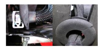
Pull back the spongy trim on the air shield. Take the rubber grommet supplied in the kit and cut a slit into it so that it can be opened up and slid over the wiring harness for the mass air flow sensor. Once it is placed on the wiring harness slide the grommet and wiring harness down the cut out on the air shield until it is in place, push the spongy trim back onto the air shield.
