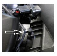
Unplug the Mass Air Sensor. Detach the Mass Air Sensor wire harness from the side of the air box by slightly pulling on the harness on the barbed mounting pin.
