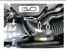
Disconnect the 3 breather hoses and the sound hose from the inlet tube. Loosen the clamps on the inlet tube at the throttle body and the air box, remove the inlet tube from the vehicle.
