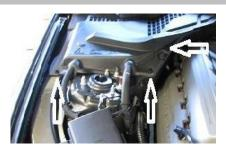
Remove the 3 screw pins that hold the battery cover to the body lift up the battery cover and disconnect the negative battery terminal.
