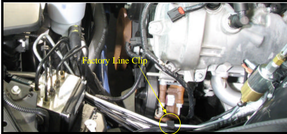
Photo 5: Proportioning Valve to Solenoid Line Routing
