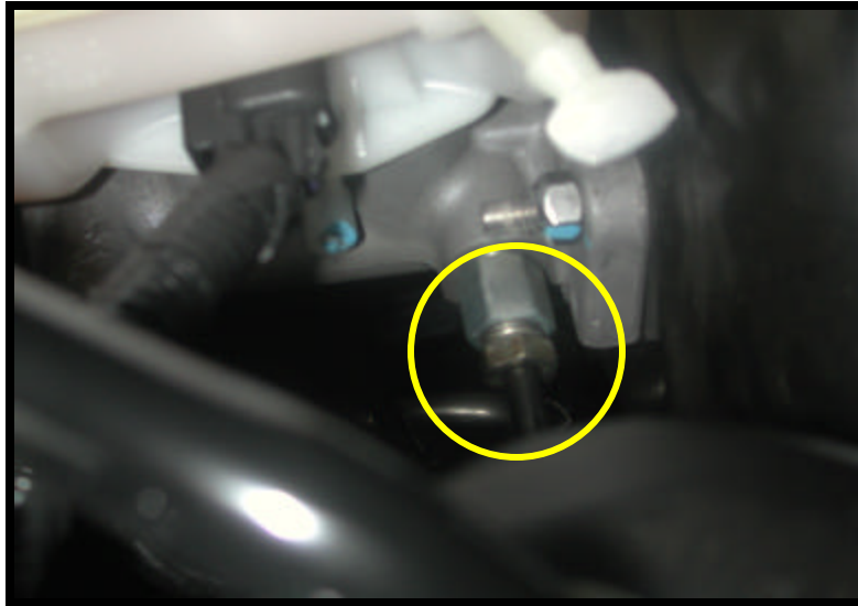
Photo 1: Location of Front Brake Line on Master Cylinder
