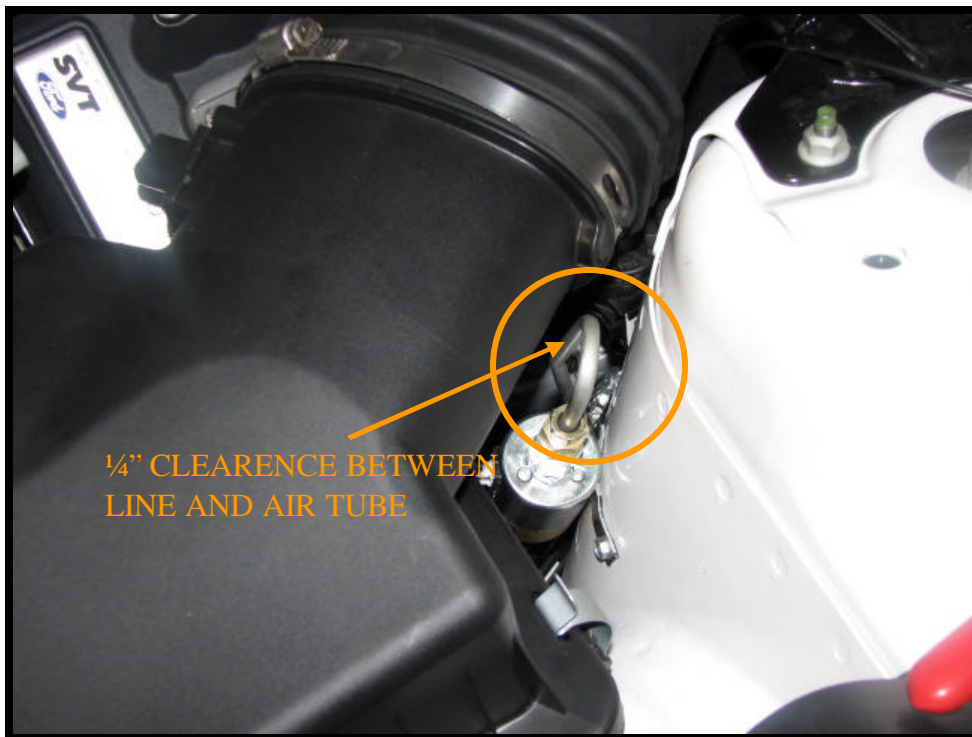
Photo 8: Line Lock Final Install Position
