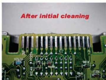
The grease and plastic must be removed
