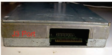
The chip will attach to the connector in the J3 Port
