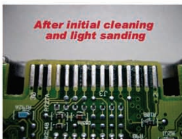
Clean the contacts and between the contacts with a Scotchbrite pad or fine sandpaper
