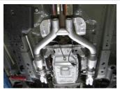
Lift the BBK H-PIPE up to the collector flanges on the headers, Connect the headers and H-Pipe utilizing the hardware supplied in the header kit. NOTE: just snug the bolts enough to hold the BBK H-Pipe into place.
