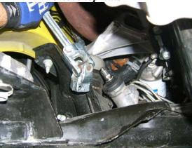
USE A RAZOR KNIFE OR GRINDER TO REMOVE THE LOCATING TABS ON THE CONNECTORS.
