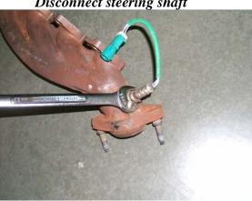
Removing the oxygen sensor
