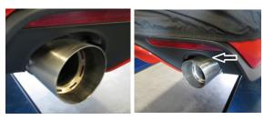
Slide the 3 " band clamp onto t the exhaust tip, then slide the exhaust tip onto the outlet tube of the muffler. NOTE!!! The bolt on the band clamp needs to be at the top with the nut facing inward towards the license plate.
