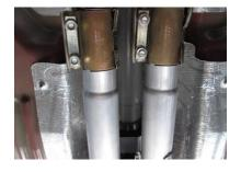
With the BBK Cat Back System install on the vehicle. Level out the BBK X-Pipe adapter and push it all the way forward towards the front of the vehicle and tighten down the stock 2 1/2" barrel clamps.
