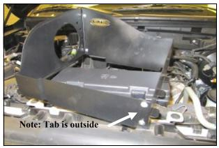
**4.** Assemble the two Quick Fit panels (#3 & #4) as shown using four 6-32 screws (#7) flat washers (#9) and kep nuts (#8).
