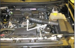
**1. Disconnect the negative battery cable!** Loosen the two intake clamps and remove the Factory intake tube.
