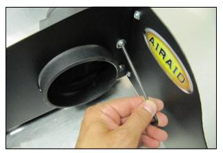
5. Install the Air Meter Tube (#2) onto the Panel Assembly and secure using the two 1/4-20 Button Head Bolts (9), and 1/4" Flat Washers (#10).
