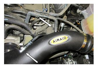
**12.** Reconnect the breather lines to the Airaid Intake Tube.
