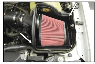
**14.** Install the Weather Strip (#8) onto the panel assembly with the contoured edge rolling away from the filter area. Start at the front of the vehicle and work your way back. Complete the installation by sliding the Airaid Premium Filter (#1) onto the Air Meter Tube and tightening the clamp.
