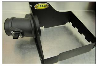
6. Transfer the MAF sensor into the Airaid Intake Tube and secure using two  $8-32 \ge 1/2$ " button head screws (#10). Do Not Use The Factory Torx Head Screws.
