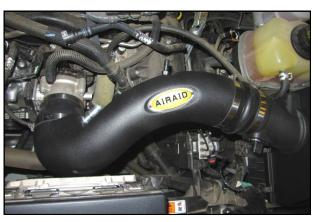
**11.** Install the Intake Tube onto the throttle body first, then into the Hump Hose. Tighten all of the hose clamps.
