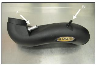
**8.** A.) Insert the 5/8" Grommet (#18) into the Intake tube as shown. Complete the tube assembly by inserting the 5/8 PCV Fitting (#16) into the Grommet. **B.)** Install the 3/8 "Hose Fitting (#20) into the threaded holt in the Intake Tube.
