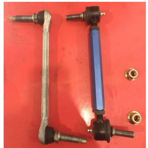
Figure 2: Factory vs Steeda front swaybar endlinks
