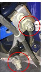
Figure 1: Factory rear swaybar endlink
