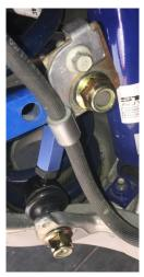
Figure 3: Steeda adjustable rear swaybar endlinks
