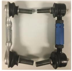
Figure 2: Factory vs Steeda rear swaybar endlinks
