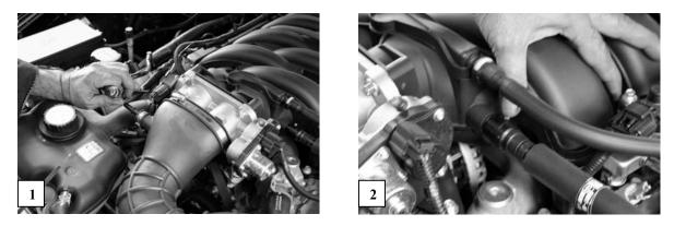
3. Remove all wiring harnesses connected to the intake manifold by pressing the release and pulling the wire from the connection. There are two connectors on the throttlebody, one on the right side for the fuel injection harnesses and one connection behind the intake manifold, next to the fire wall for the actuator motor. **Figure 3**
