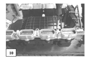
15. Install the new Charge Motion Delete Plates with the four Torx screws removed in Step 14. Note that there are left and right sides, with the left side marked "LH" and the right side marked "RH". The gasket groove in the new Steeda Charge Motion Delete Plates should be visible with the spot-face/nitrous ports facing each other. Take care to align the new plates so they fit the O-rings around the intake ports as well as match the injector ports. **Figure 11**
