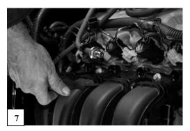
12. Once the bolts are removed, carefully lift the intake manifold from the engine and place on a workbench away from the engine. It is a good practice to cover the intake ports with shop towels until you are ready to reinstall the intake. This will help prevent debris from falling into the engine.
