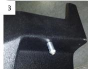
8. Remove the factory air intake sensor. This is located in the factory lid facing forward. Simply rotate it counter clockwise to remove. Use the supplied rubber grommet (smaller OD) and install the grommet into the forward facing hole in the Steeda CAI base. Then using a twisting motion install the sensor as shown. See figure 5.
