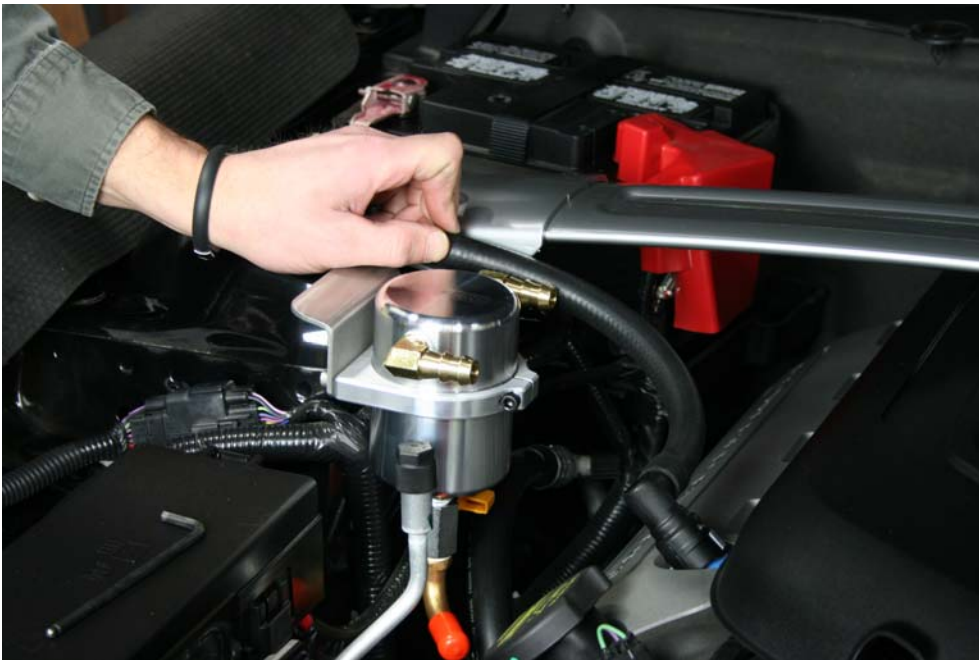
Step 20: Route 1/2" hose from valve cover to rear fitting of Air Oil Separator and mark for trim cut
