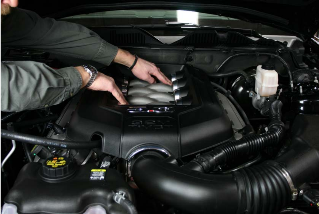
Step 10: Re-Install Intake cover
