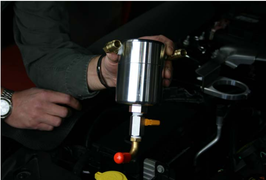
Step 15: Assemble Air Oil Separator as shown, apply Teflon tape to all fittings
