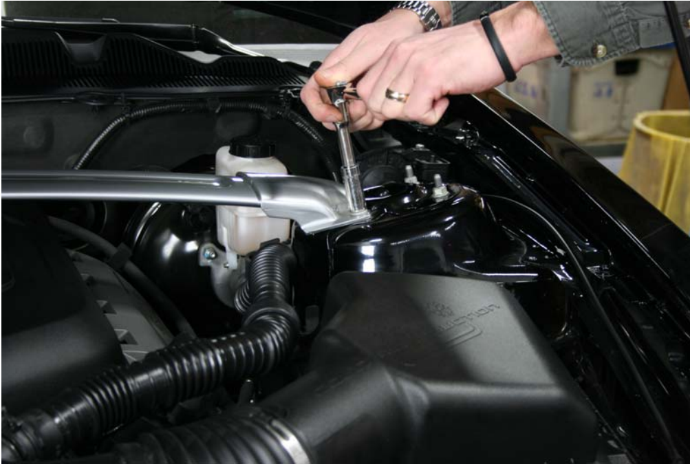
Step 14: Re-Install all mounting bolts
