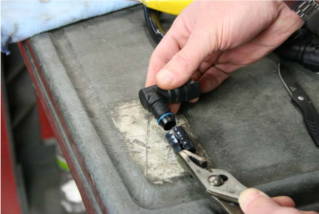
Step 6: Remove remaining tube from 90 degree fittings and set 90 degree fittings aside
