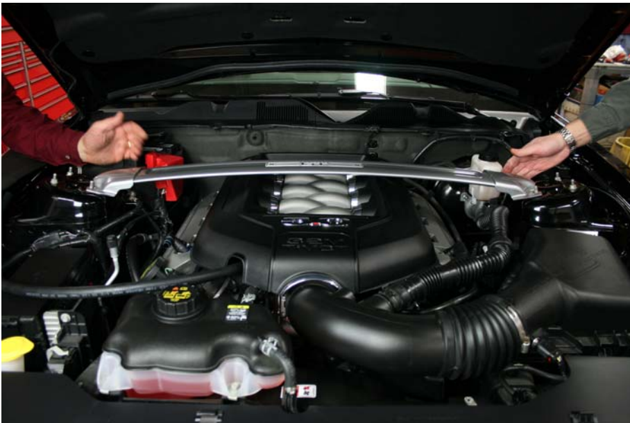
Step 11: Re-Install Strut Tower brace
