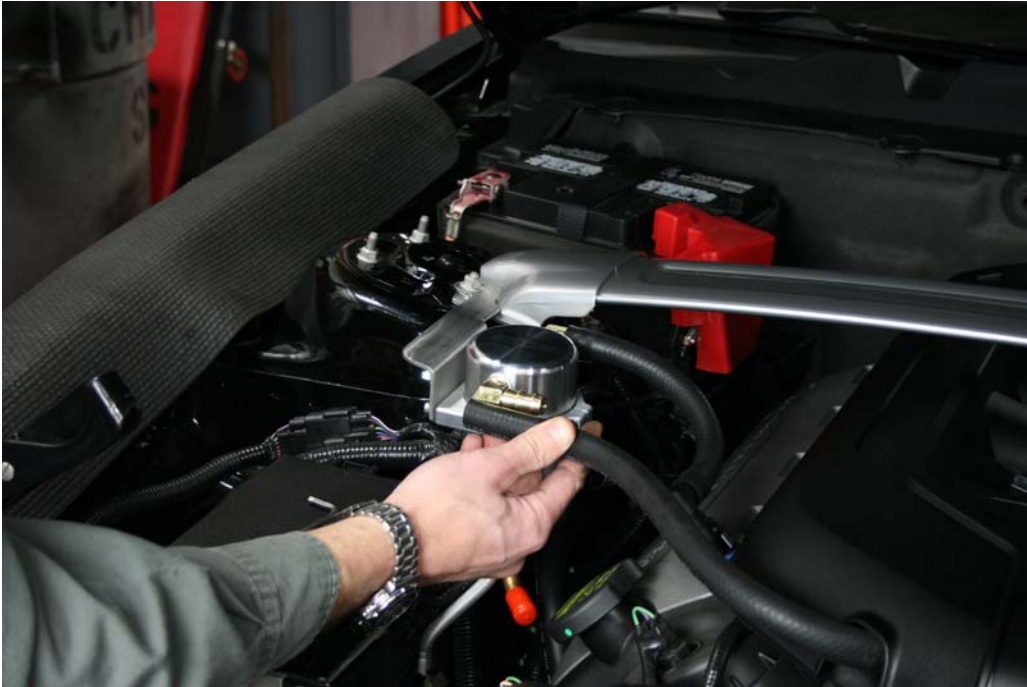
Step 22: Route 1/2" hose from intake to front fitting of Air Oil Separator and mark for trim cut
