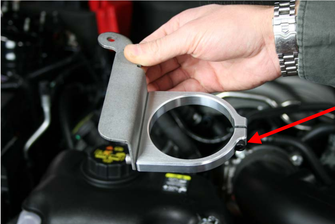
Step 12: Assemble Billet mounting bracket to stainless mount, note orientation of 1/4x20 SHCS
