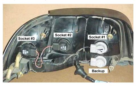
3) Remove the sockets from the tail light fixture using a counter-clockwise twist. Pull the light bulbs out of the sockets, and place the bulbs into the new harness. (NOTE: If your car is 3 years old or older, it might be a good idea to replace the bulbs while the fixtures are off the car.)
