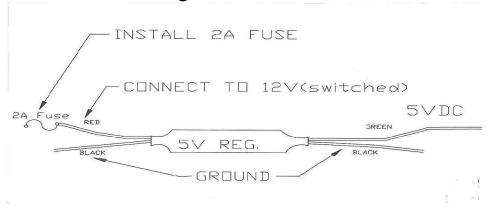
RED-----SWITCHED 12VDC (Use a fused circuit or "Add-a-Circuit" available at most auto parts stores for easy and clean installation)
